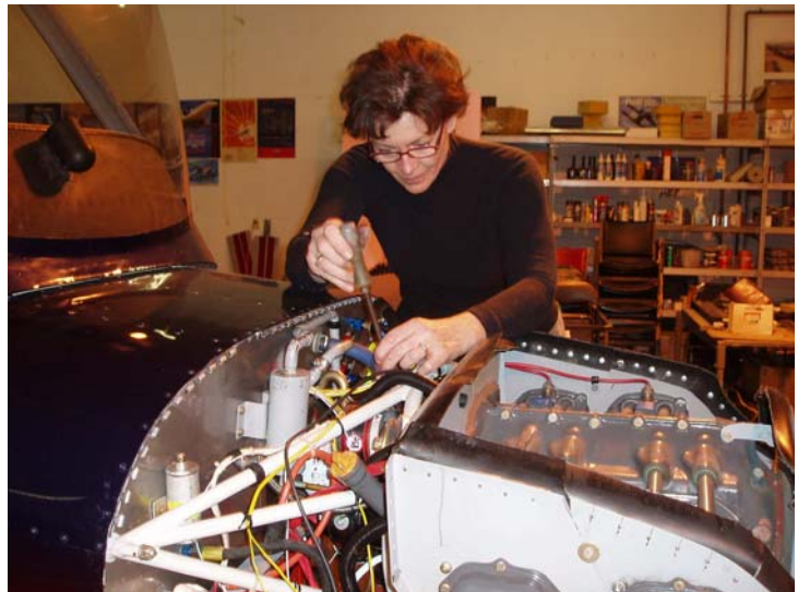
'Getting to the Oil Filter' for the '50 hour' Oil Change On Bravo Juliet Juliet'
