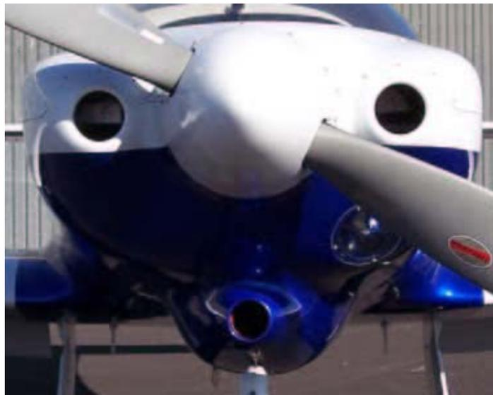
Figure 1, Induction Air Inlet
